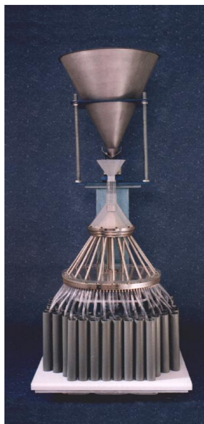
Figure 3: Sample Sub-division by Spinning Riffler
