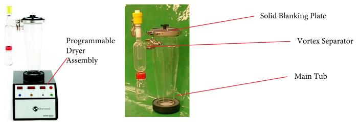
The vertical chamber (tub) is designed to allow air in at the bottom and flow upwards. Air flow out the top of the main tub is inhibited by the presence of a solid blanking plate. The side collection vessel has a vortex separator. in which particles flowing from the main tub hit the central tube in the vortex separator and drop to the bottom of the collection vessel.
