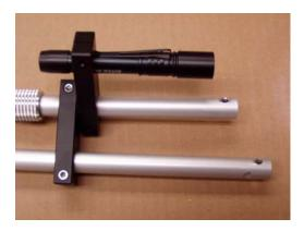
10. Insert the lower end of the adjustable angle adapter into the top end of smallest tube, align the pin holes on the tube and the lower end of the adjustable angle adapter, and lock the assembly by inserting the ball spring pin into the aligned holes.
