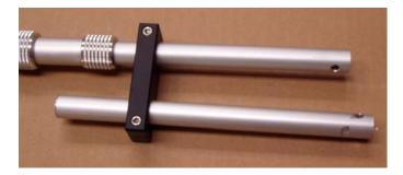
8. Mount the second Delrin adapter, through the lower hole, on the extended end of the smallest tube and tighten the lower screw on this Delrin adapter.
