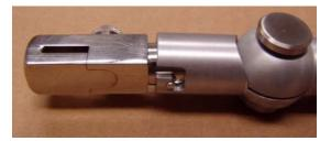
12. Adjust the angle of the adjustable angle adapter by loosening the thumb screw tilting the top part of the adjustable angle adapter to the desired angle and locking it in place by tightening back the thumb screw.
