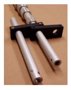
9. Remove the end cap of the flash light, insert the rear end of the flash light through the upper hole of the second Delrin adapter, replace the end cap and tighten the upper screw of the Delrin adapter. The flash light may be turned on or off by tightening or loosening the end cap.
