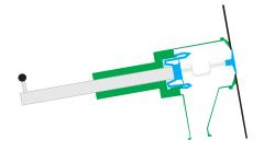
The FreeGlide will work with pipes that are up to  $10^{\circ}$  from vertical
