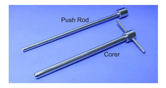
Method of Construction: Crevice free, all welds ground and polished
