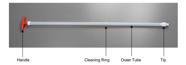
Diameter of Outer Tube: 25mm
