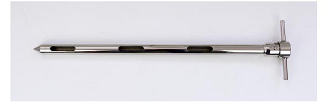
Method of Construction: Surface Finish: **Overall Length:** Outer Tube Diameter: Number of Sampling Ports: Position of Sampling Ports: Welds ground and polished Better than 0.8 microns Ra (product contact surfaces) 600mm 25mm 3
