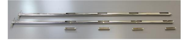
Method of Construction:Fully weldedFinishExternal Bright Polished<br/>Internal Machine finishNominal Length:2050mmDiameter of Outer Tube:40mmNominal Weight of Sampler:6.6 KgNo. of Sampling Slots4 offPosition of Slots:4
