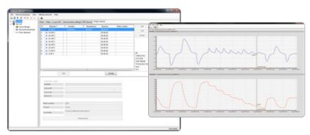
Fully automatic aw measurement can be planned if the AwTherm is connected to the HW4 software. The instrument then moves to preset temperature points automatically and carries out a pre-selected Aw Quick or Aw Equilibrium measurement.
