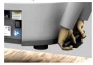
You can also use the transport lock for lifting the device with a crane.
